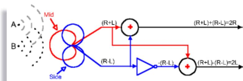
The MS Decoder performs sum and difference operations to extract Right and Left level and phase information from the Mid and Side signals. In the illustration the circles with "+" signs represent summing functions.
